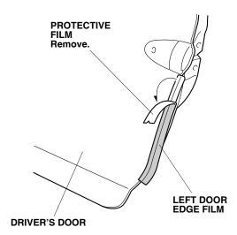
7. Starting from the top and working downward, use the soft sleeve to fold the left door edge film inside the driver's door as shown.
