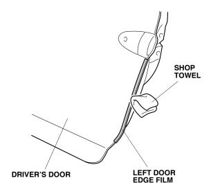
9. Repeat steps 1 through 8 to install the door edge film on the right side of the vehicle.
