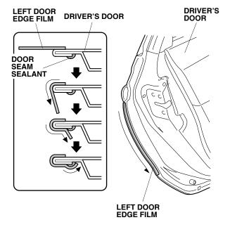
Using a shop towel, wipe the excess 3M protective tape application solution from the left door edge film.
